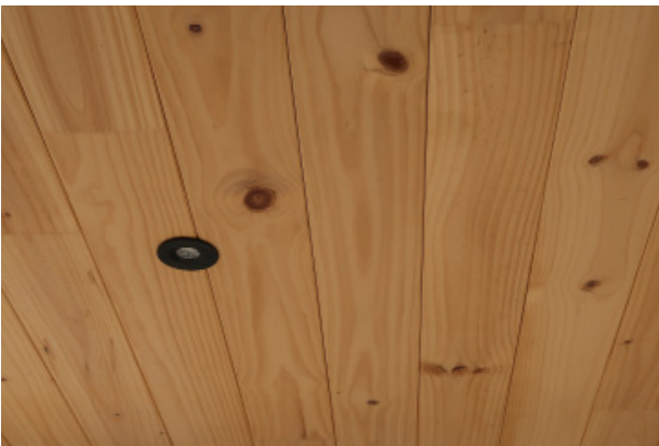
A typical XLam Natural Appearance Grade surface.
