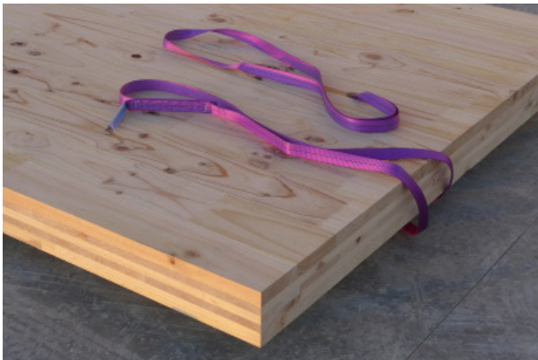
Factory-threaded webbing sling ready for lifting.
