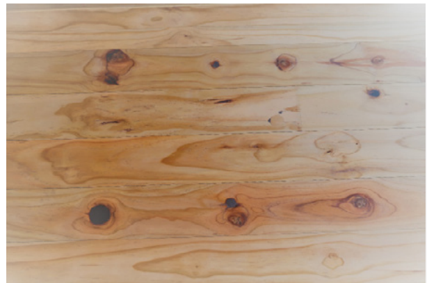
Dark fillers blend with the overall surface appearance.
