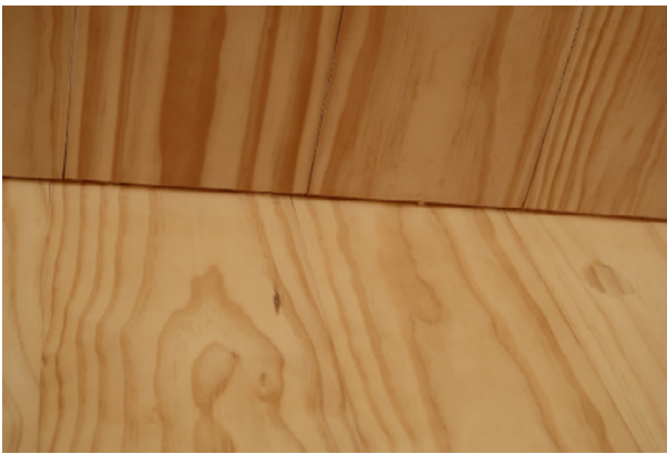
Carefully selected plugs will blend with the surface.
