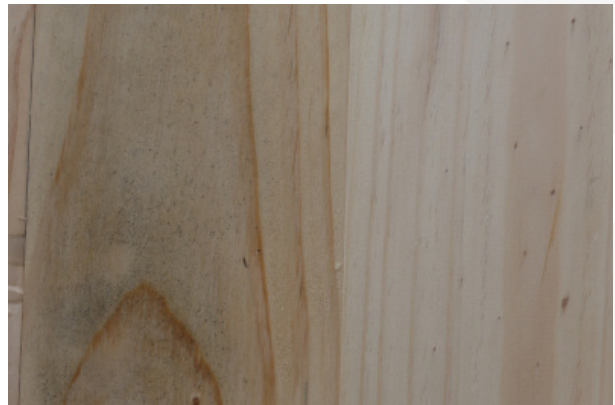
Surface mould spores developing under a polythene cover.
