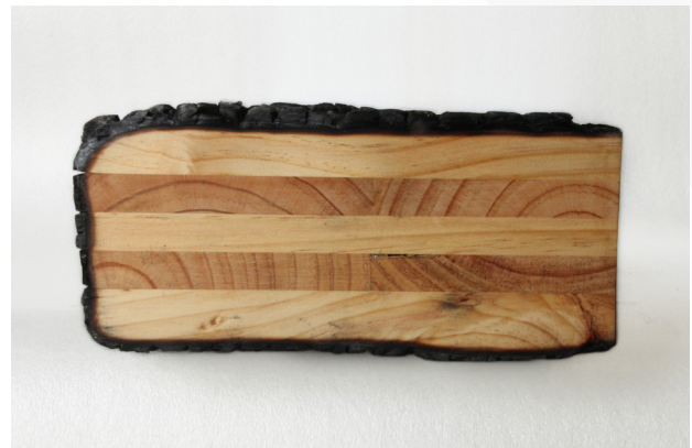
Sample cut from an unlined XLam intermediate floor/ceiling, still structurally intact after total building burnout.
