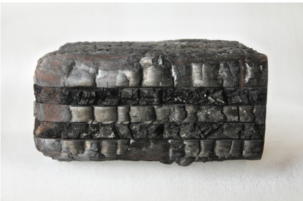
Sample cut from an unlined XLam intermediate floor/ceiling, still structurally intact after total building burnout.
